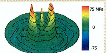
Stresses in an optical fibre preform
